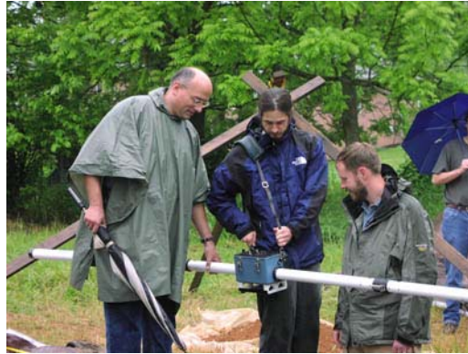
Dr. Rhett Herman demonstrates the use of the EM-31 Electromagnetic Conductivity Meter in archeological investigations.
