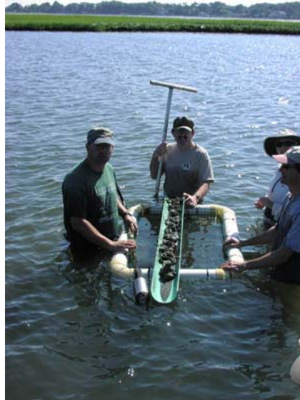
Phil King, NRCS Soil Scientist (on left) demonstrates collection of a Subaqueous soil core using a bucket auger.
