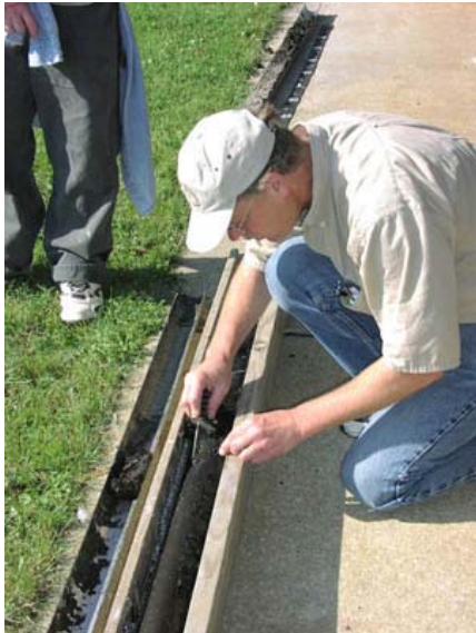
Dr. Mark Stolt (U of RI) prepares to describe a soil profile collected with the vibracore rig.
